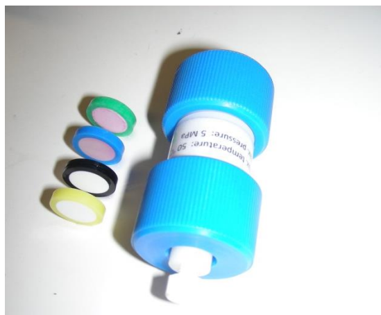
Figure 11. CIM® disks and housing. CIM® disks (left) are white monoliths placed in the middle of the disk of a non-porous self-sealing ring with different colors according with their ligand chemistry. CIM disk is inserted in the CIM housing (right) and used as a chromatography column.
